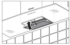
6) If you plan to have a tiled backsplash or wall panel underneath the exhaust hood, this may cause difficulties when changing the filter, depending on the thickness and height of the tiles or panel.
